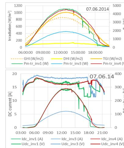
The performance is affected by partial shading, which is a typical challenge for building implemented systems in urban areas. As an example, the figures to the left show (top) irradiation and AC power and (bottom) DC current and voltage curves for three arrays (inv1, inv3, inv4) during a clear summer day.
