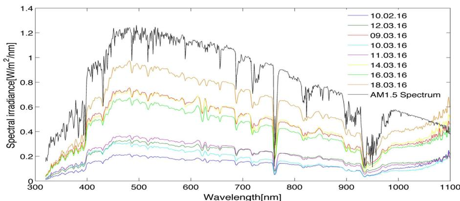
**Figure 1:** Measured solar spectra at Kjeller and in Grimstad vs the AM 1.5 solar spectrum. The solar spectra presented are the ones with the highest spectral irradiance from each sequence.
