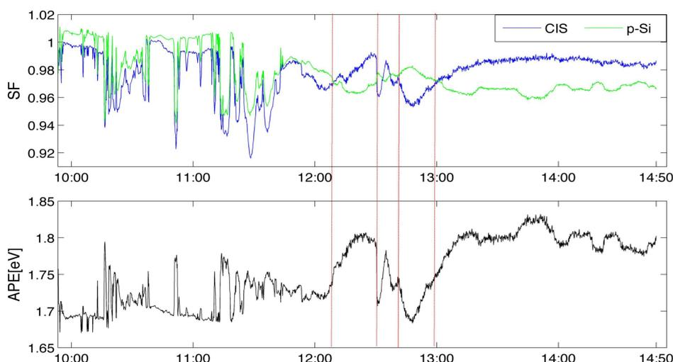
**Figure 3:** The combined figures show the correlation between average photon energy (APE, **bottom**) and spectral factor (SF, **top**) of both modules, and how it varies during the day. The calculated values are based on 1769 measurements performed on the 18.03.16 at Kjeller. The red lines indicate some of the regions when the spectral factor of the two different modules deviates.
