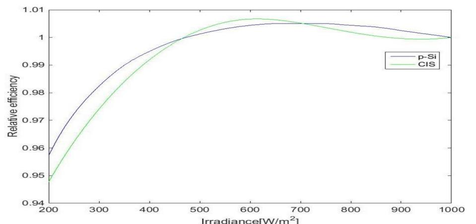
**Figure 5:** Relative efficiency with respect to irradiance levels, for both the CIS- and p-Si module. The average efficiencies of the CIS- and p-Si modules at light intensities 400-500 W/m<sup>2</sup> are 13.37 % and 15.88 %, respectively. The p-Si module is produced by IBC SOLAR and has a STC efficiency of 15.9 %. The CIS module is produced by Solar Frontier and has a STC efficiency of 13.4 %.
