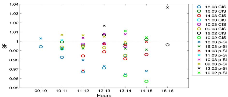
**Figure 2:** The daily variation in spectral factor (SF) for every measurement sequence. The spectral factor indicates the performance of the considered solar module under the actual spectrum relative to the performance under the standard 1.5 AM spectrum. The presented SF values are average values of calculated spectral factors based on each measurement conducted during each hour.
